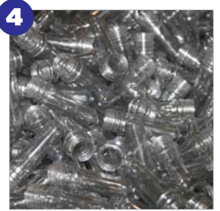
4 Preformed bottle blanks are fed into a hopper.
