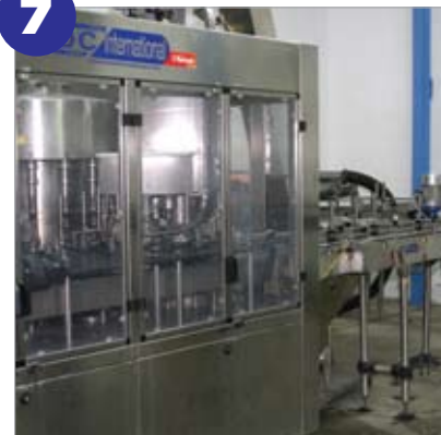
7 The washed bottles are filled with spring water in a sterile environment.
