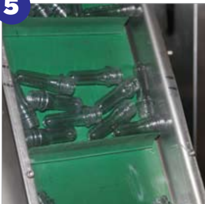
5 Bottle blanks travel to the blower which extrudes them into an 8-oz. or 16-oz. bottle.
