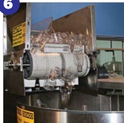
6 Formed bottles exit the blower and are thoroughly washed.
