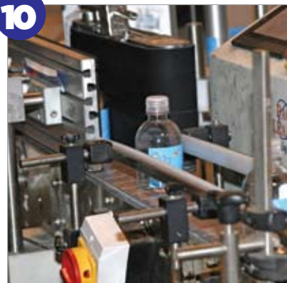
10 Bottles travel through the label applicator and are placed into cases.
